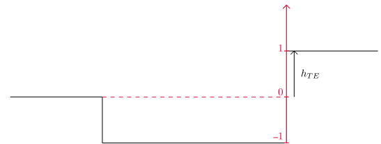
Fig. 5 The design variable, h_{\text{TE}} , for the open deep cavity.
